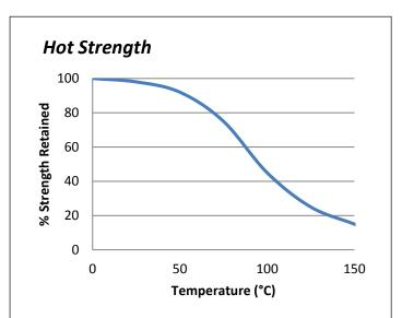
"Hot strength" shear strength tests performed on mild steel. Fully cured then conditioned to pull temperature for 30 minutes before testing. MS359 CLEAR can withstand higher temperatures for brief periods (such as for paint baking and wave soldering processes) providing the joint is not unduly stressed. The minimum temperature the cured adhesive can be exposed to is -40°C (-40°F) depending on the materials being bonded.
