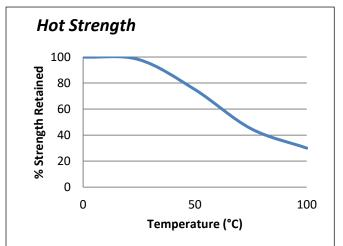
Fully cured lap shear specimens conditioned to pull temperature for 30 minutes before testing at temperature.
