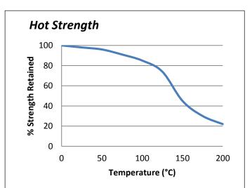
"Hot strength" shear strength tests performed on mild steel. Fully cured then conditioned to pull temperature for 30 minutes before testing. ES564 can withstand higher temperatures for brief periods (such as for paint baking and wave soldering processes) providing the joint is not unduly stressed. The minimum temperature the cured adhesive can be exposed to is -40°C (-40°F) depending on the materials being bonded.
