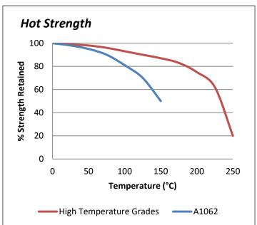
"Hot strength" Breakaway strength on M10 steel bolts according to ISO 10964. Cured at 23°C for 24 hours then conditioned for 30 minutes at testing temperature.
